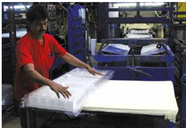
One of Megapac's staff manually arranging the packaging for cutting on an old machine
